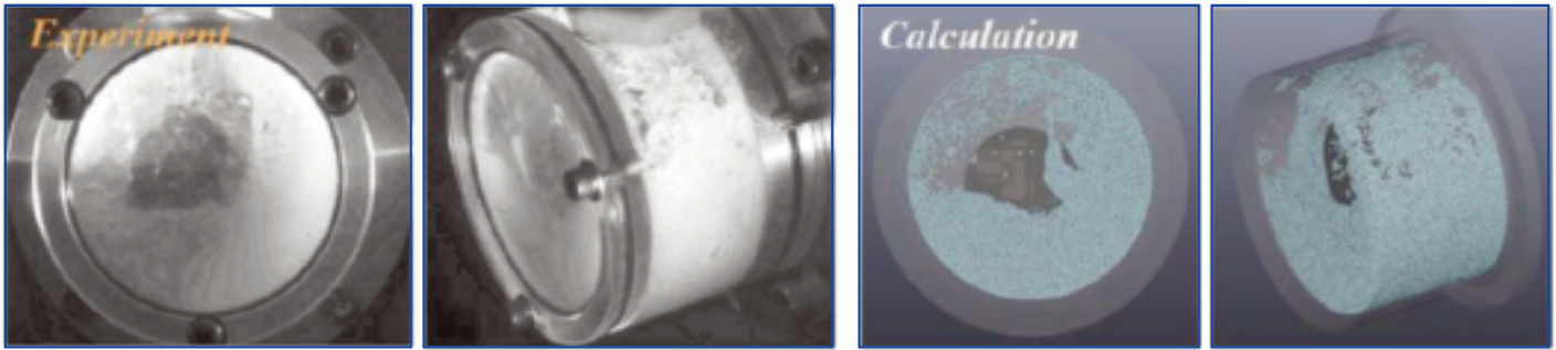
Figure 2: Oil circulation in a crankcase (1,750rpm)
