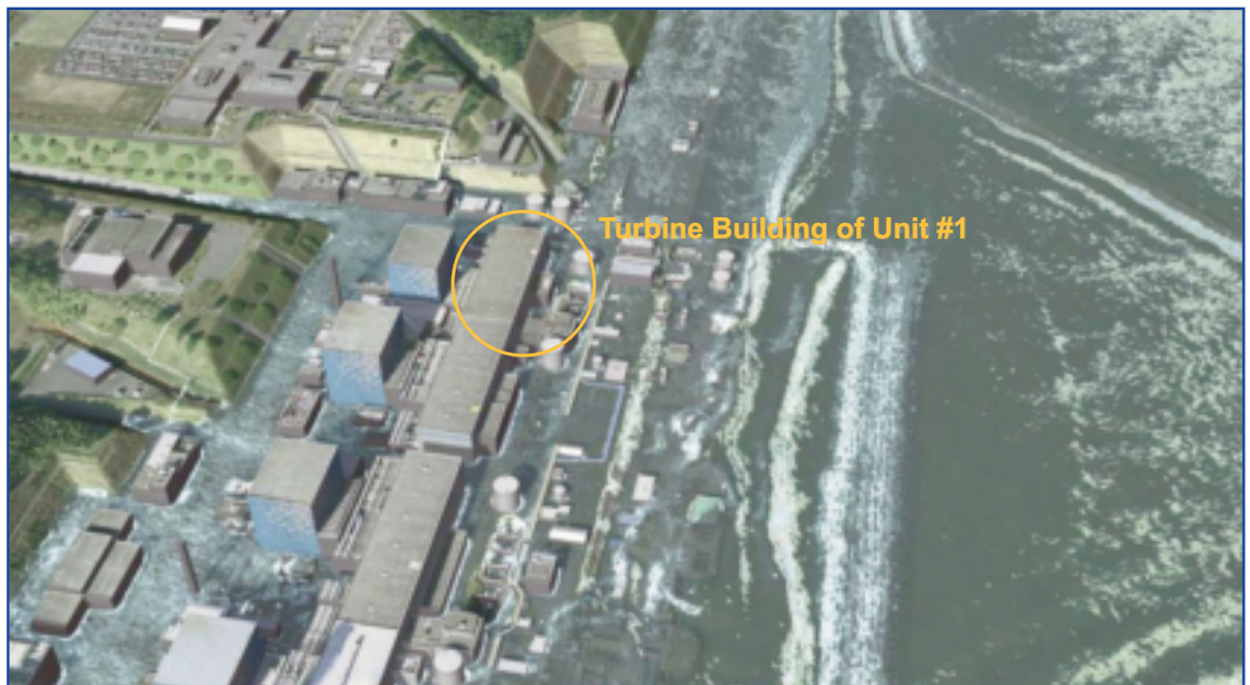
Figure 6: Three-dimensional tsunami run-up simulation on Fukushima Dai-ichi Nuclear Power Plant by the Great East Japan Earthquake in 2011
